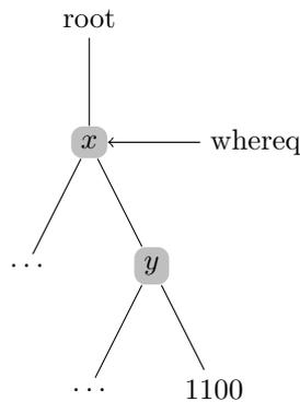
Here we wish to remove 1100, however if we left its parent with a single child pointer, that would make the parent nothing more than a bump in the road - it should also be removed. Thus we need a pointer to the grandparent in order to remove both the string and the internal node that pointed to it.
